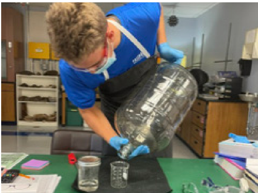
Aidan, prepping the chemical reaction: 2C_3H_8O + 9O_2 \rightarrow 6CO_2 + 8H_2O .
